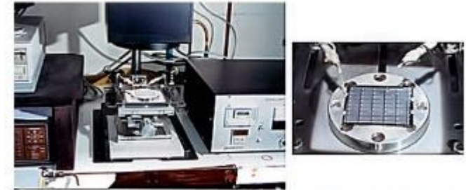
The standard solar simulator used for testing the efficiency of the thin film solar cells.
